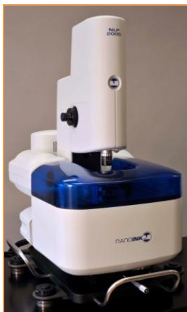
Figure 1. The desktop nanolithography platform NLP 2000 TM was used for patterning hydrogels.
